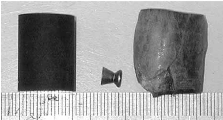
**Fig. 1.** Lipari rhyolite cylinders used in our experiments. Left: an unheated, unimpacted control sample. Centre: unused “diablo” airgun pellet. Right: sample that was heated to 900°C and then shot with airgun pellet. This caused impact vesiculation throughout, but especially in the region closest to the where the pellet struck (the left-hand edge as seen here). Scale bar is graduated in mm.
